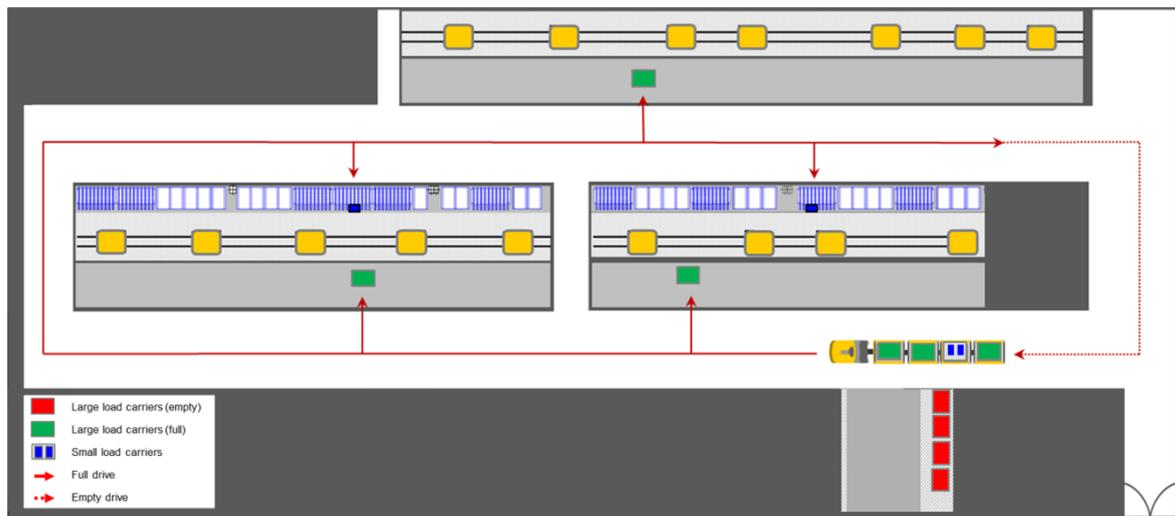
Figure 6: New process with tugger train delivery
