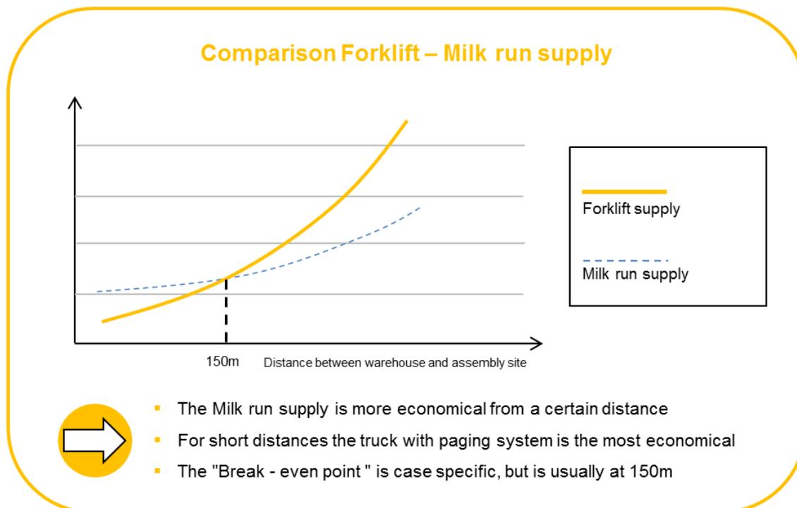
Figure 5: Comparing fork lift delivery and tigger trains
