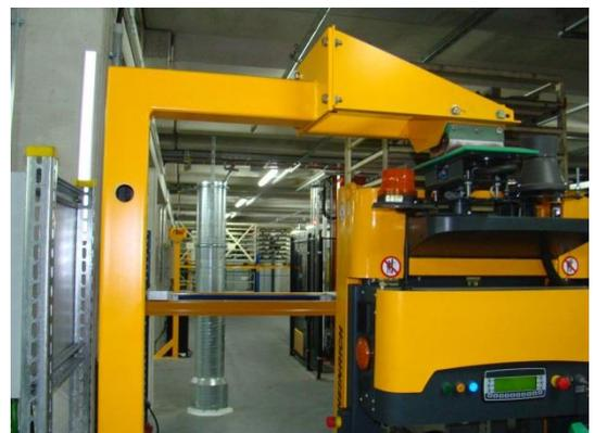
eration in order to compensate for the charging time. As the recharging time is only 10 minutes, a different recharging station is not needed for each vehicle. The reference point here is one recharging station for 3 APM vehicles.
