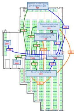
The Jungheinrich WMS and Logistics Interface map the warehouse's logistic processes and control material flow in accordance with the defined processes. For this, material flow is first analysed, and then modelled for the warehouse management system and stored in WMS as strategy. This is the starting point for the process logic of the "Truck Guidance System" module in particular.
