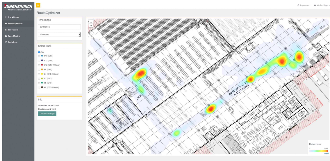
Image 4: Visualization of the trucks' movement inside the warehouse, module RouteOptimizer. The heatmap helps recognize which routes are used by most trucks, thus revealing the potential for optimizing transport routes.
