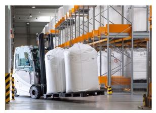
RX 60 counter balanced trucks move the bulk bags to the rack system.
