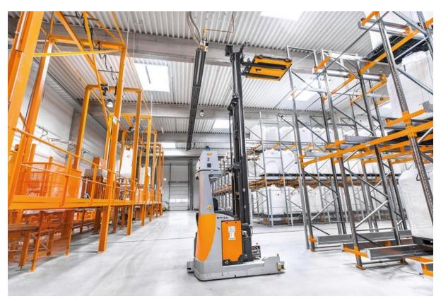
For the first time STILL implemented the interplay of semi-automated shuttles with fully automated FM-X reach trucks in a channel rack.
