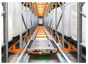
A shuttle retrieves a pallet to supply production.
