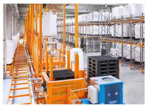
Perfectly harmonised interaction of the conveyor equipment with the transfer carriage and the stacker for empty pallets.
