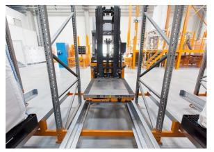
To retrieve the bulk bags the FM-X reach truck places the shuttle precisely to the millimetre in the right channel.
