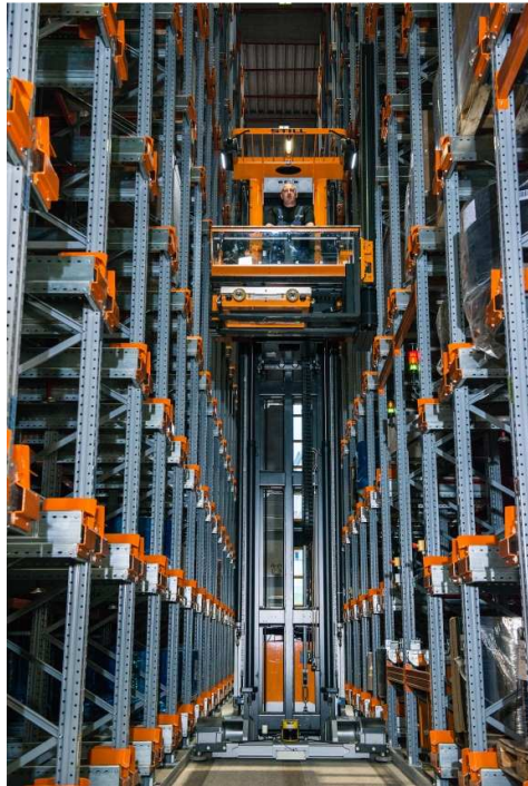
Figure 2: Pallet shuttle high rack warehouse (18 metres) with space for 10 650 palettes
