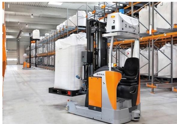
The FM-X reach trucks automatically move the bulk bags to the conveyor equipment on the working platform.
