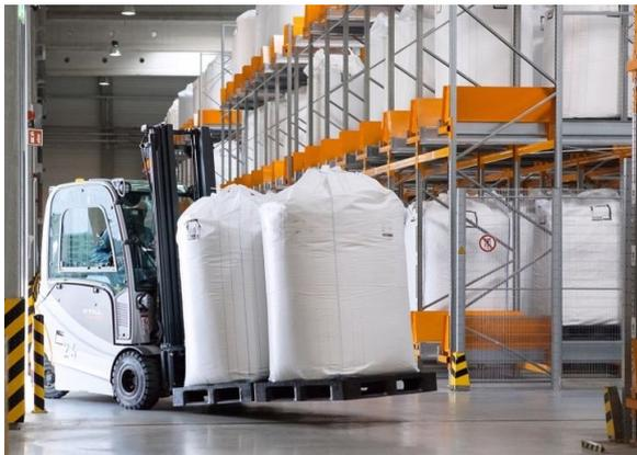
RX 60 counter balanced trucks move the bulk bags to the rack system.
