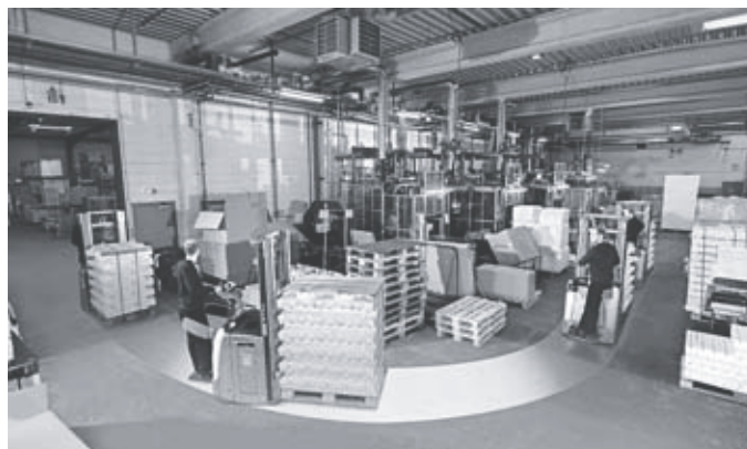
Safe even when cornering: automatic speed reduction around corners
