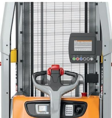
Large touch screen at eye level for intuitive operation and maximum ease of use
