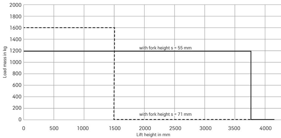
1. This diagram shows the loads and shelf heights for which the automated truck can transport, store and retrieve loads safely, reliably and consistently.
