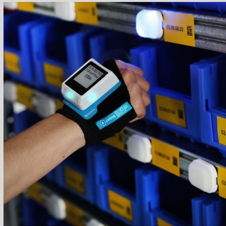
**EASY PAIRING** - the LIGHT TAG and the corresponding storage location are scanned and finally paired
