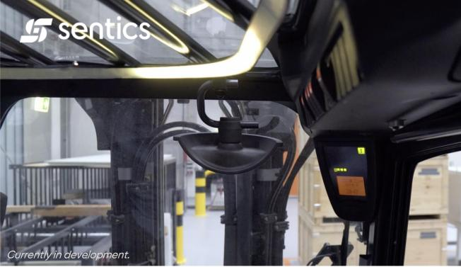
In this case, an approach is shown with a yellow colour. If the distance between the truck and the person becomes smaller, a critical distance is marked in red. If the distance is reduced further, the system flashes to achieve the greatest warning effect.
