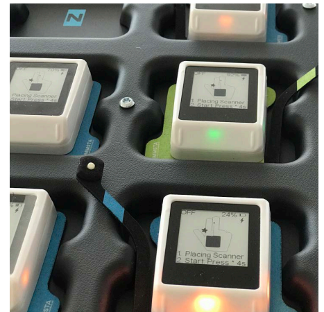
WIRELESS CHARGING - LOAD STATUS AT HS 50
