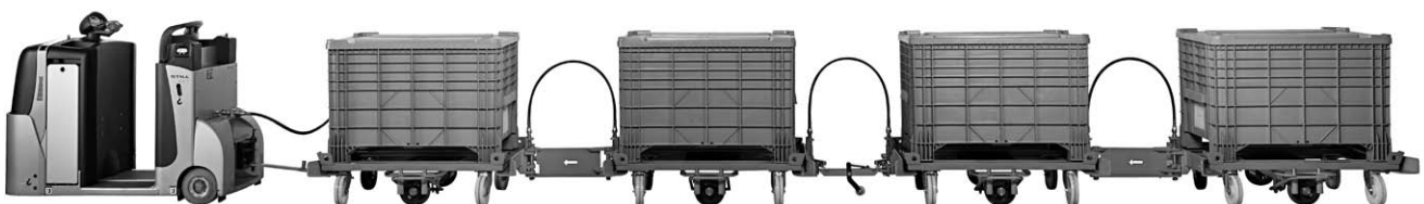
E-type frame with independent system and articulated tiller
